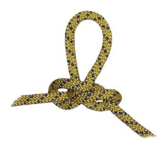
Designed at the request of our customers, this rope is intended for use as a bagged throw rope for boat or shore based water rescue. The continuous stranded polypropylene core provides flotation to the wear – resistant braided nylon sheath. This rope has a higher breaking strength than economy polypropylene water rescue rope, and is much easier to grip.
