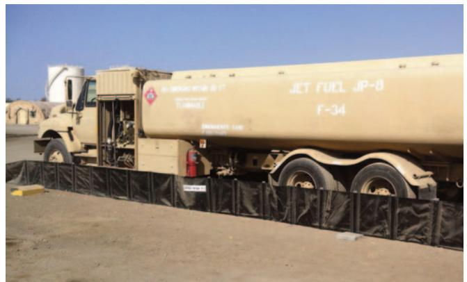
(Based on 30 oz. per square yard material) (The standard berm material is XR-5 8130 unless otherwise specified)
