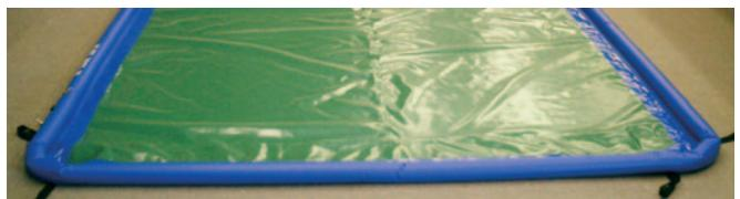
Husky air wall berms have a continuous air chamber that allows the air to disperse throughout the chamber when driving in and out of the berm. This design, along with the pressure relief valve, eliminates blowouts.
